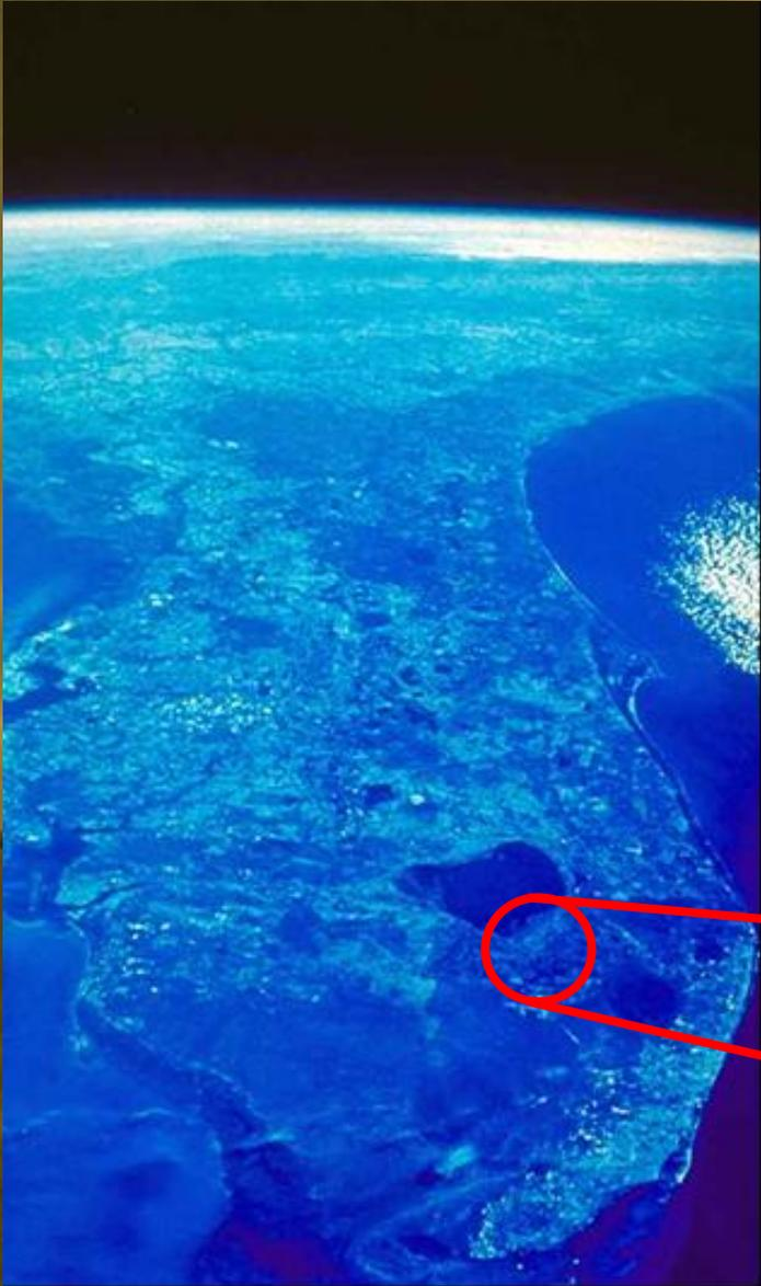
**Stormwater Treatment Area 3/4 is the world's largest constructed wetland! Over 16,500 acres of former agricultural land has been converted to a biological treatment system designed to remove over 55 tons per year of phosphorus from water entering the Everglades.**
