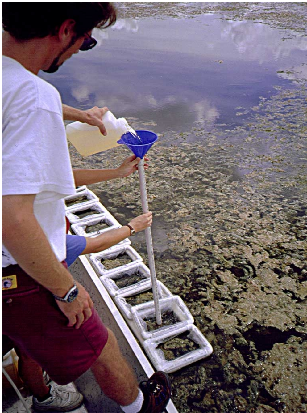
Figure 6-41. Field crew spiking microcosms with inorganic P solution during an experiment of P uptake by the Ceratophyllum /periphyton complex. During each experiment, the microcosms were suspended at the top of the water column by floating PVC pipe frames and left open to the atmosphere. Microcosms were filled with marsh water and a quantity of plant material collected from the immediate area.
