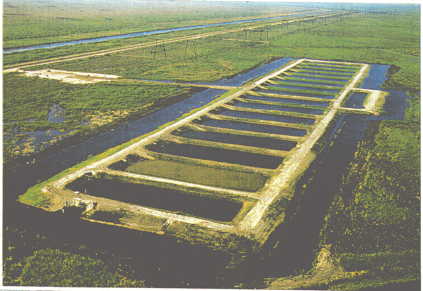
TWO SETS OF 15 RESEARCH CELLS WILL BE USED TO EVALUATE THE EFFECT ON NUTRIENT-REMOVAL PERFORMANCE OF VARIABLES SUCH AS HYDRAULIC LOADING RATES, NUTRIENT LOADING RATES AND PLANT DENSITY. EACH CELL IS ABOUT THE SIZE OF A FOOTBALL FIELD.
